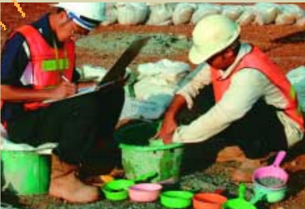
Geologists logging drill cuttings
