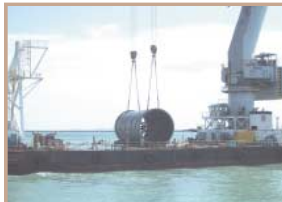
Transferring SAG mill shell to dock at Lam Chabang port, Thailand
