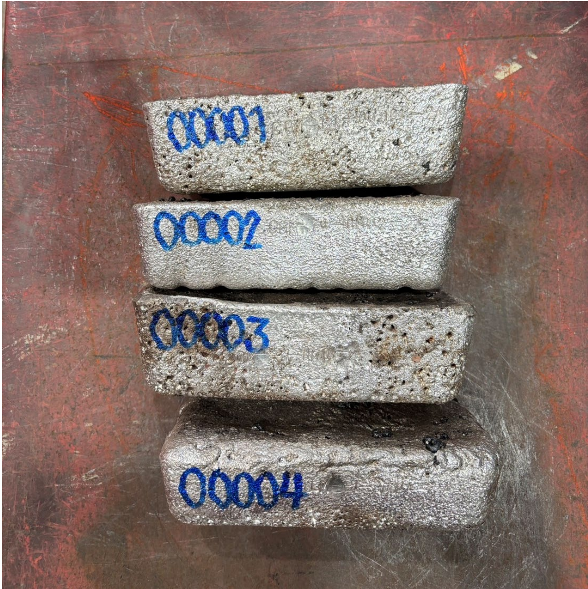
The first four doré bars poured at Chatree Gold Mine on 6 June 2024
