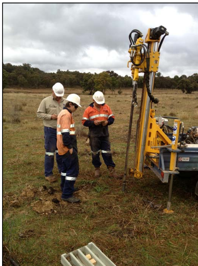
Testing topsoil depths and geochemistry, Bowdens Silver Project
