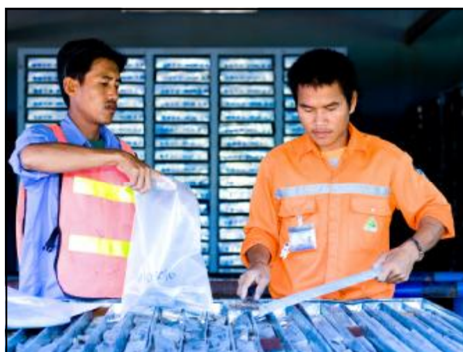
Pracha Laophet and Nueng Kanthong collecting diamond drill core samples
