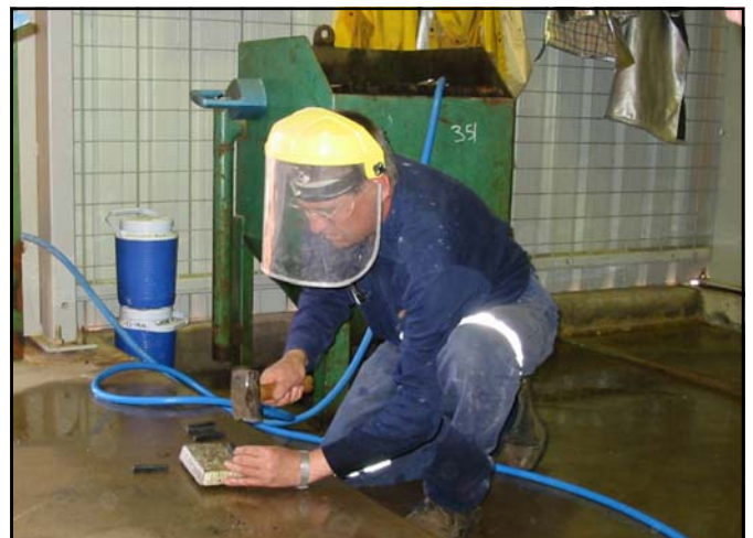
Stamping the ID numbers into a recently poured Challenger gold bar.
